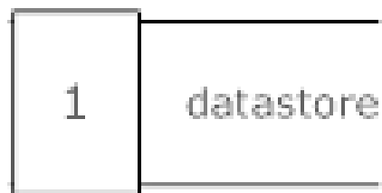
figure 6: the data store in data flow diagrams [4]
